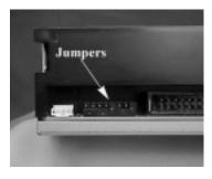
The block of mode select jumpers are located on the rear of the DVD-ROM. If the jumper covers both pins on the jumper block, it is ON; if there is no jumper or only one of the pins is covered, the jumper is OFF. The jumper settings include SCSI ID, Parity, Termination, Eject, Test/Audio Playback, and Power Supply.
